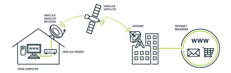
Satellite internet access works just like satellite TV (e.g. DStv) and operates according to the same technology;
