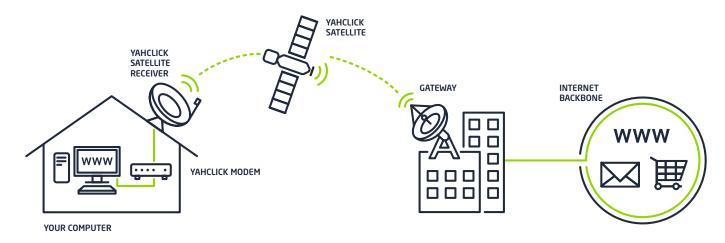
Satellite Internet access works just like satellite TV (e.g. DStv) and operates according to the same technology;
