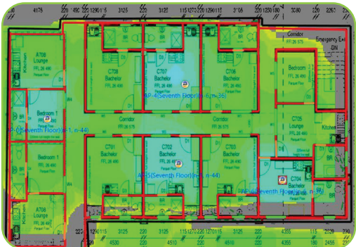
RF Heat Map example (indicating AP placement and Wi-Fi coverage)
